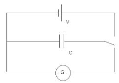
First close the key in the upper position to charge the capacitor from the power supply of the known potential difference, V. Then move the key to the low position to discharge the capacitor through the galvanometer and measure the deflection of the galvanometer, d. (Once again do it twice switching polarity and then take the average of the two readings). In this case the charge is  $\Delta q = CV$ , so
