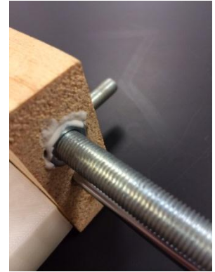
Figure 4. Block and screw system that is attached to the stepper motor that moves sensor platform.
