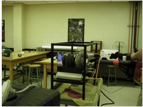
Even though the engine was not able to stay in a stable working mode for long periods of time due to insufficient airflow from the leaf blower, it has been a definite success showing that such a thing as jet engine built out of scrap materials is even possible. It now belongs to the
